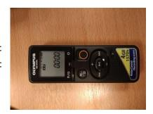
2. Slide REC switch on to record the introduction to the test session. The indicator light turns red.
