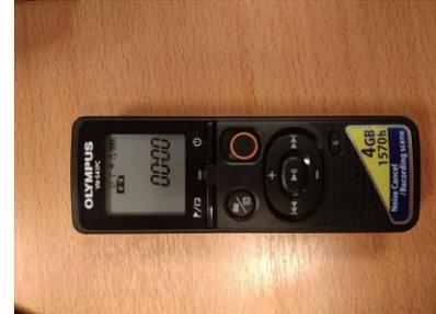
2. Slide REC switch on to record the introduction to the test session. The indicator light turns red.
