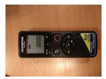
2. Slide the REC switch ( ) on to record the introduction to the test session. The indicator light will
